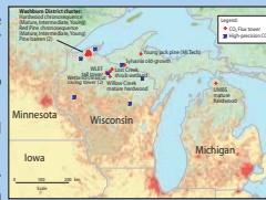
Fig 1. MODIS land cover map of region showing locations of eddy covariance towers (red cross) and summer 2004-2005 CO 2 tracer deployment (blue stars).
