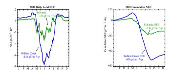
Daily and cumulative total net ecosystem exchange (NEE) of CO<sub>2</sub> in 2002 for Sylvania and Willow Creek as measured by eddy covariance flux towers. Sylvania annual NEE was -136 gC/m<sup>2</sup>; Willow Creek annual NEE was -438 gC/m<sup>2</sup>. Missing data are filled using fitted functions of soil temperature to respiration (R) and PAR to gross ecosystem production (GEP = R-NEE).
