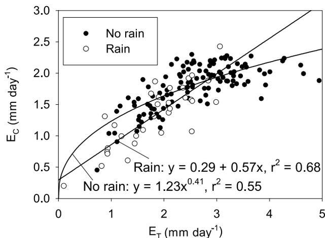
**Figure 5.** Comparison of daily sum of transpiration ( $E_C$ ) upscaled from sap flux measurements and total evapotranspiration ( $E_T$ ) measured with the eddy covariance method on days with and without rain. A power curve fits the data without rain, and a linear curve fits the data with rain.
