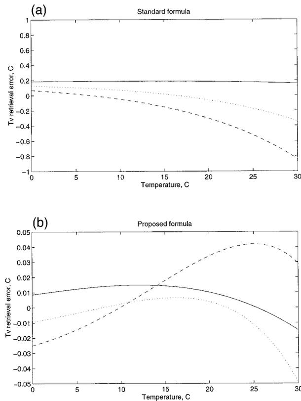
FIG. 6. (a) Error in retrieval of RASS virtual temperature using the standard formula (1) compared to the formula of Cramer (1993). The solid line is for 0% relative humidity, dotted line 50%, and dashed line 100%. (b) Error in retrieval of RASS virtual temperature using (2) compared to the formula of Cramer. Line types indicate relative humidity as in (a). Note that the vertical scale is reduced by a factor of 20 from (a).
