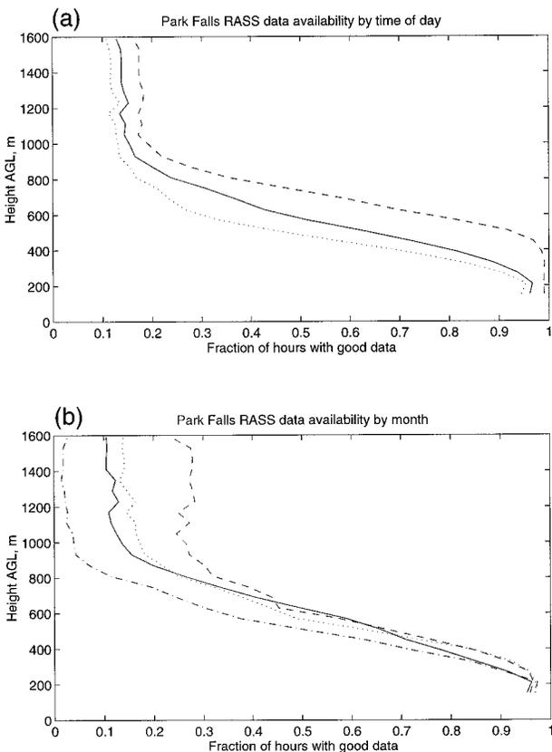
FIG. 2. Height coverage of RASS virtual temperature measurements. Line types are as in Fig. 1.
