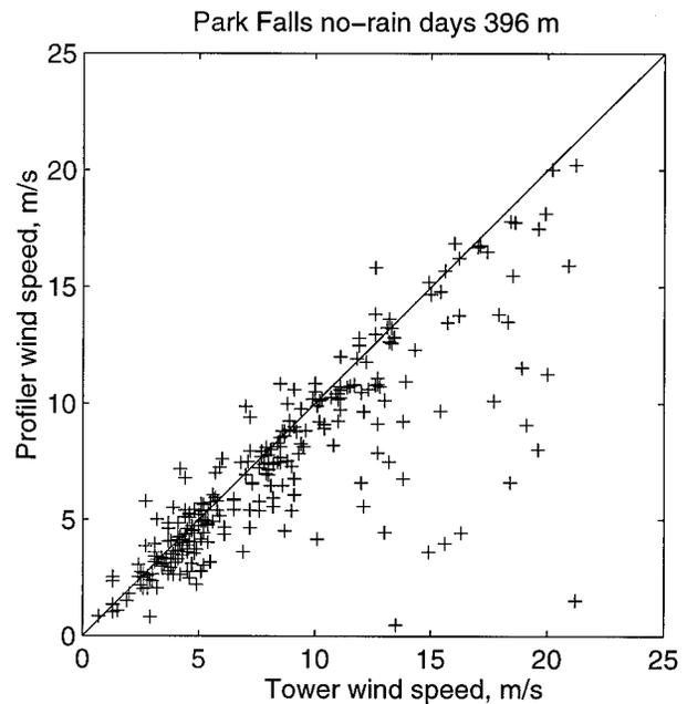
FIG. 3. Scatterplot of hourly average wind speed from the profiler vs the tower anemometer. The solid line is 1:1. Two hundred sixty-five points are included.
