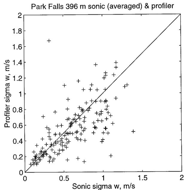
FIG. 9. Vertical velocity standard deviation on resolved scale only from profiler vs sonic anemometer. See text for computation details. The solid line is 1:1. Hourly values for 167 h are included.
