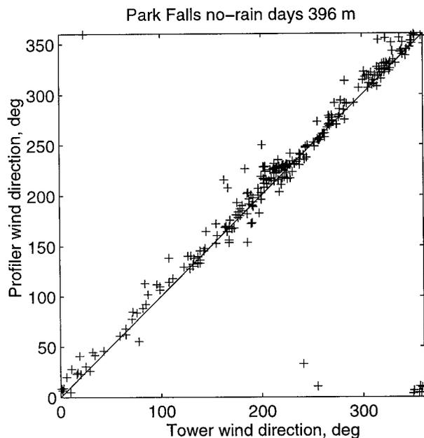
FIG. 4. Scatterplot of hourly average wind direction from the profiler vs the tower wind vane. The solid line is 1:1. The same 265 points are included as in Fig. 3.
