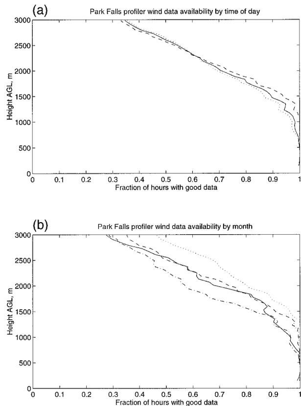
FIG. 1. Height coverage of profiler winds. (a) By time of day. Solid line is for all hours, dashed line for daytime (0800–1700 LST), and dotted line for night (1700–0800 LST). (b) By month. Solid line is for June, dashed line for July, dotted line for August, and dash-dot line for September.
