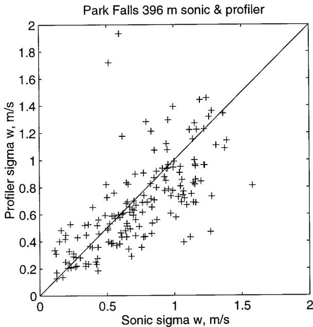
FIG. 8. Vertical velocity standard deviation on all scales from profiler vs sonic anemometer. See text for computation details. The solid line is 1:1. Hourly values for 167 h are included.
