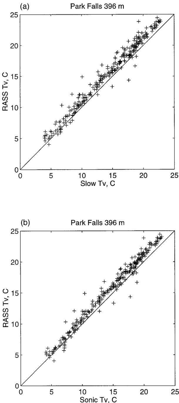
FIG. 5. Virtual temperature from RASS vs tower sensors. (a) Slow thermometer/hygrometer. (b) Sonic anemometer. The solid line is 1:1. The 250 points are 6-min averages at the beginning of each hour.
