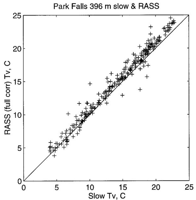
FIG. 7. Virtual temperature from RASS with turbulence, displacement, and retrieval corrections vs tower slow sensor. The solid line is 1:1. The same 250 points are included as in Fig. 5.
