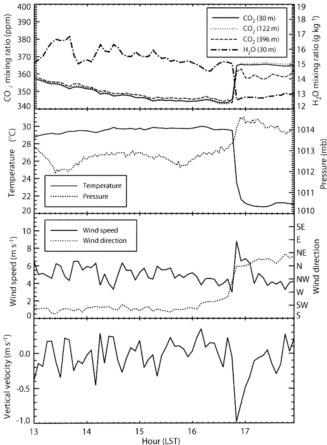
FIG. 5. Atmospheric changes at the WLEF tower on 14 Jul 1998 during a frontal passage. The frontal passage occurred at 1645 LST. All data shown were recorded at the 30-m level except for CO<sub>2</sub>, for which 122- and 396-m data are also shown. Data are 5-min averages.
