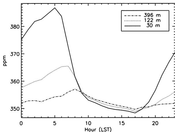
FIG. 1. The average diurnal cycle of  $\text{CO}_2$  mixing ratios at 30, 122, and 396 m at WLEF during Jun–Aug 1997.
