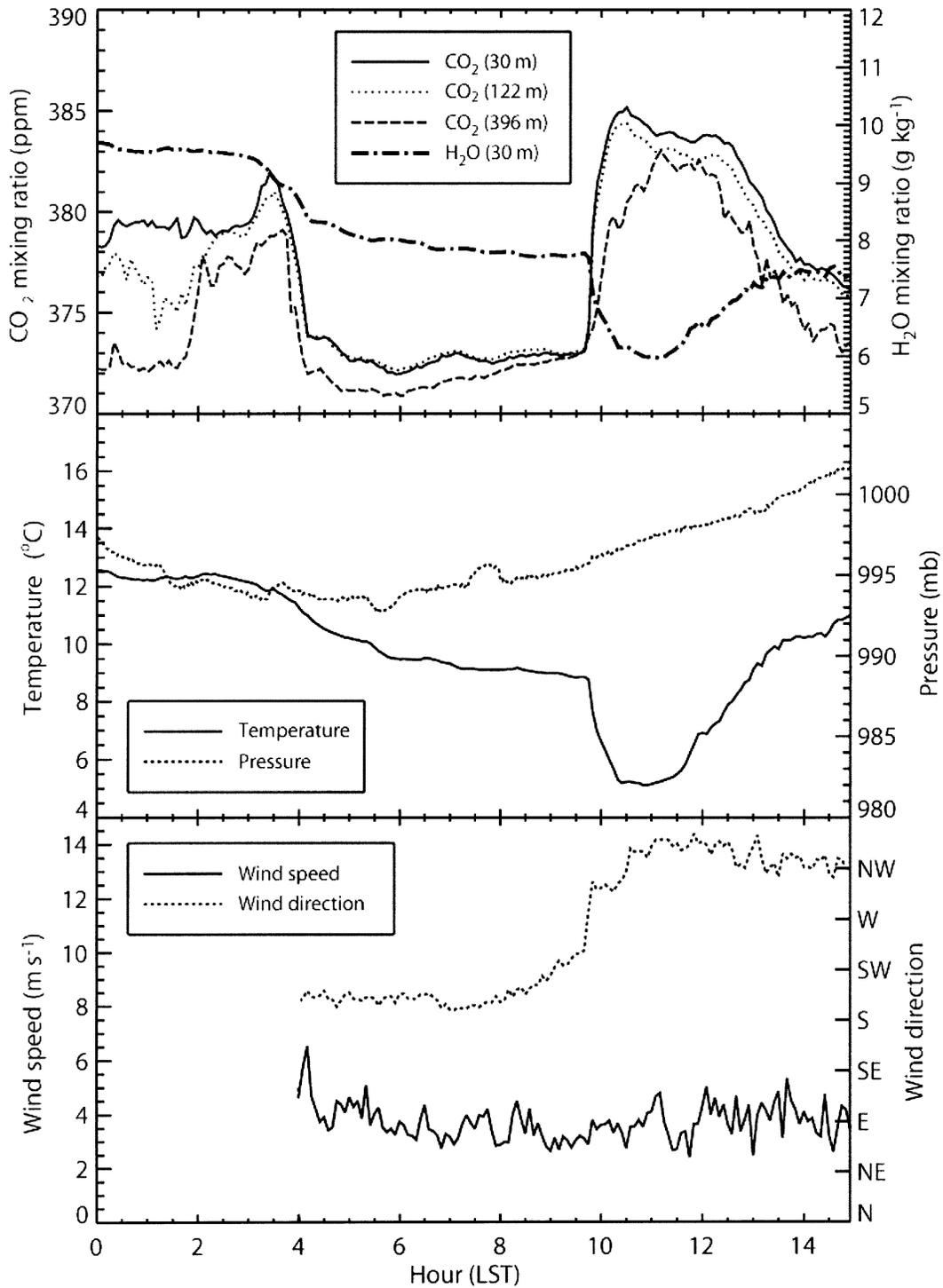
FIG. 8. Atmospheric changes at 30 m at the WLEF tower on 28 Mar 1998, in which horizontal and vertical transport phenomena are explored. All data shown were recorded at the 30-m level except for CO<sub>2</sub>, for which 122- and 396-m data are also shown. Data are 5-min averages. Wind speed and direction data were not available before 0400 LST due to instrument failure.
