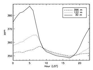
FIG. 1. The average diurnal cycle of  $CO_2$  mixing ratios at 30, 122, and 396 m at WLEF during Jun–Aug 1997.
